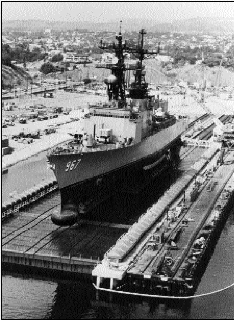
U.S.S. ELLIOT, a “Spruance” Class Destroyer, on the Syncrolift® at Todd Pacific Shipyards Corporation, Los Angeles Division (Note that the vessel has been docked on a special high cradle which allows both the propeller and bow sonar dome to clear the platform during transfer.) Syncrolift® Platform dimensions: 655ft. x 106ft. (199.6m x 32.3m); maximum lifting capacity: 22,200 long tons.
